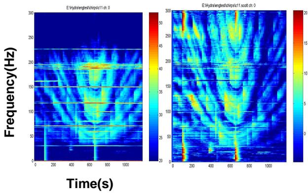
Fig.10. Spectrogram for a single phone as the source passed over the Hydra array before (left) and after (right) pre-whitening.
