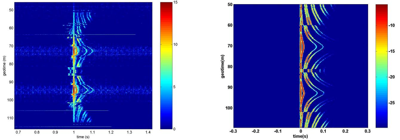
Fig.7.Measured(left)andmodeled(right)channel impulse response as the source is towed over the array and back again
