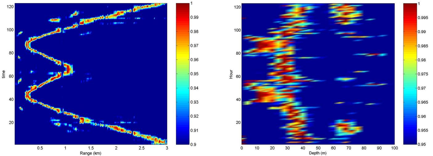
Fig.8. Range-time (left) and depth-time tracking derived by correlation processing on a single phone.
