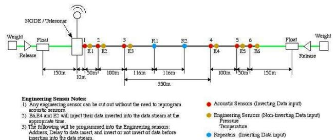
Fig. 2. Configuration of the Hydra array.
