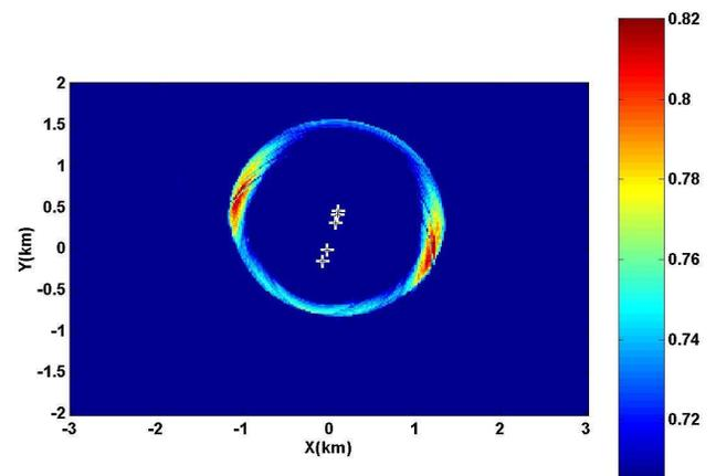
Fig.9. Range/cross-range snapshot generated by correlation processing of multiple phones.
