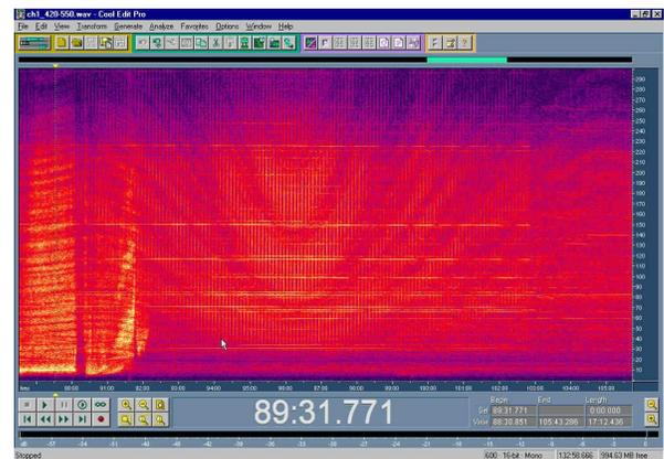
Fig.6. Spectrogram of one of the Hydra channels during an overpass by the towship.
