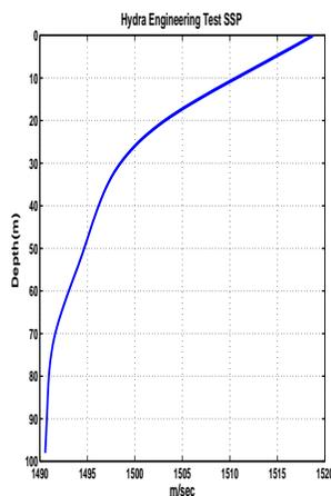
Fig.4. Sound-speed profile measured during the Hydra Sea Test.
