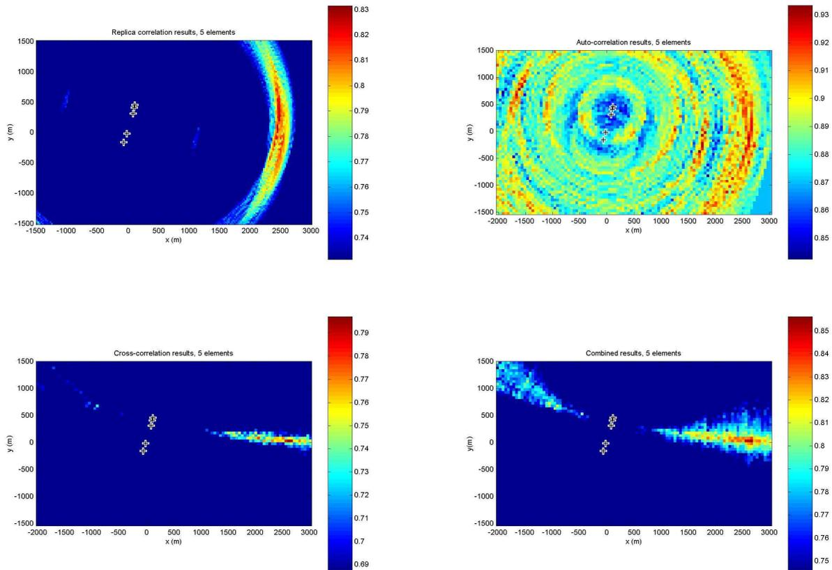
Fig.13. Ambiguity surfaces generated via a) Replica correlation, b) Auto-correlation, c) Cross-correlation, and d) Auto-and cross-correlation.
