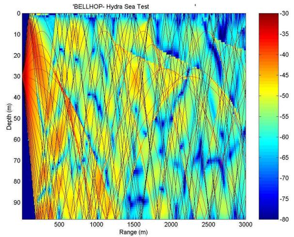
Fig.5. Ray-traces superimposed on transmission loss for the test site.
