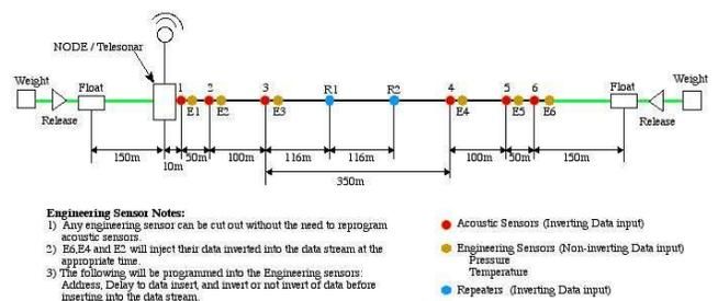
Fig. 2. Configuration of the Hydra array.
