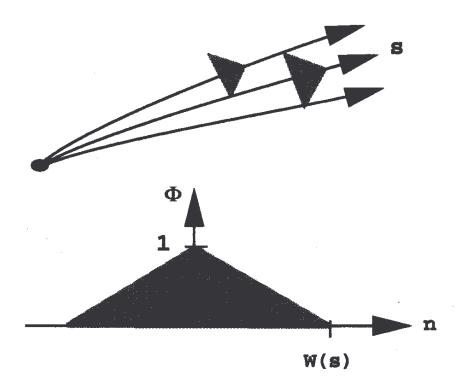
Figure 1: Construction of a finite-element ray.
