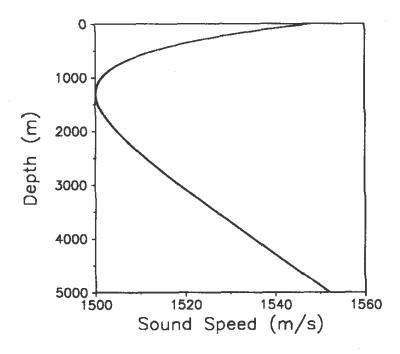
Figure 2: Sound speed plot for the Munk profile
