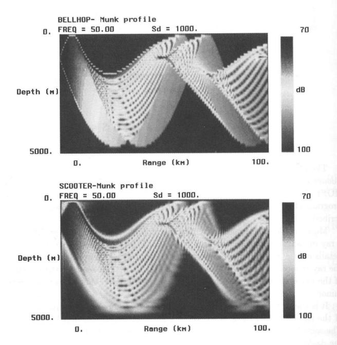
Figure 4: Transmission loss for the Munk profile using the FER method (upper) and an FFP program (lower).
