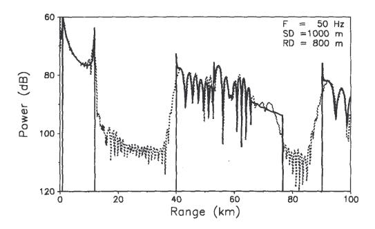
Figure 5: Transmission loss for the Munk profile for a receiver depth of 800 m using the FER method (dashed) and an FFP (solid).
